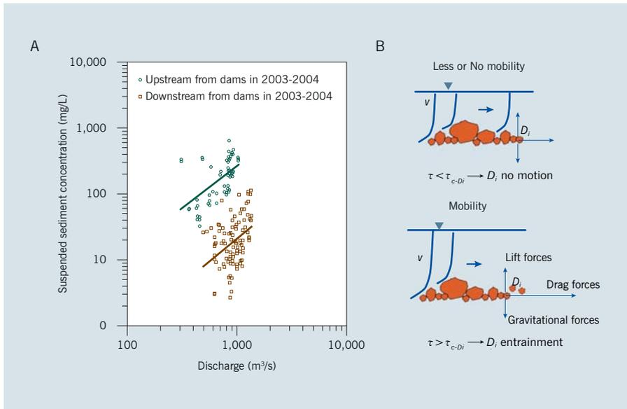
Note:  $v$  = flow velocity,  $D_i$  = particle of an  $i$  diameter,  $\tau$  = shear stress,  $\tau_{c-Di}$  = critical shear stress for a given particle size  $i$ .
